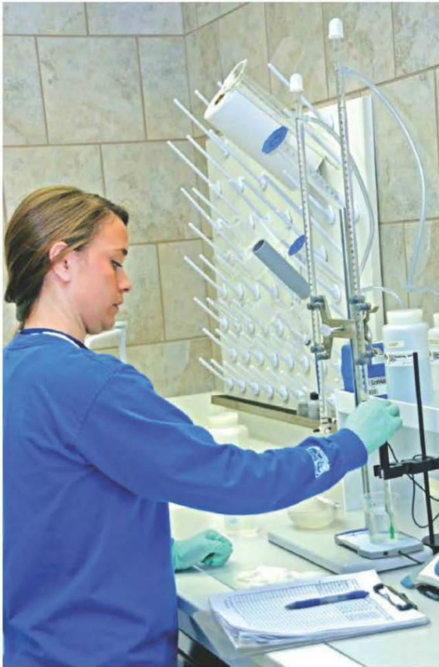
Senior laboratory technician Alison McGee conducts a total alkalinity test.
